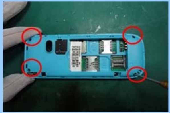
2. Unfasten the 4 screws by screw driver
